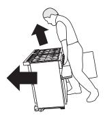
Do not use the door handles or control knobs to manoeuvre the cooker. Use the hotplate and griddle bowl areas.
